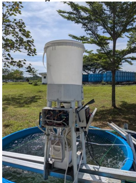
Figure 4. Physical implementation of the automatic feeder unit
